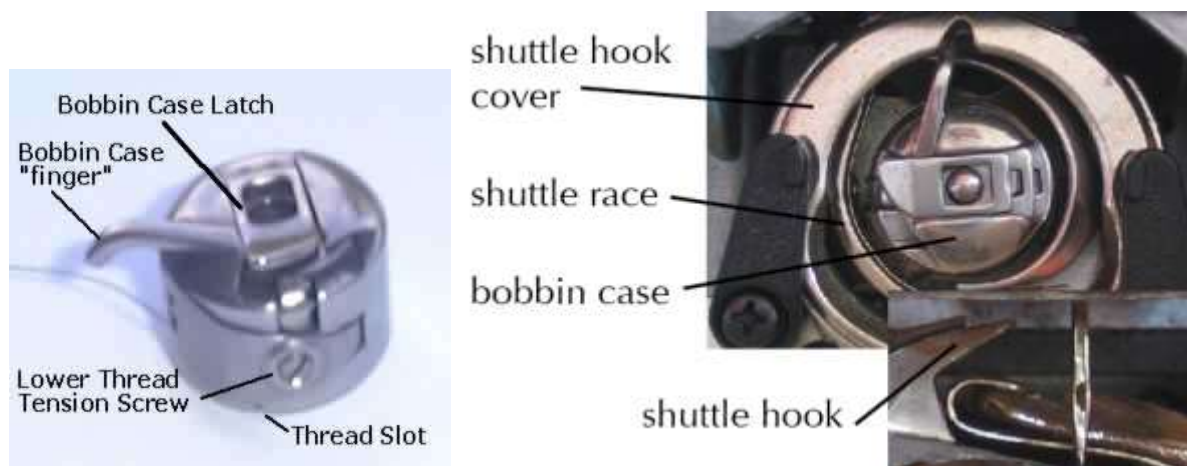
Fig 5: 2 bobbin case and shuttle block
